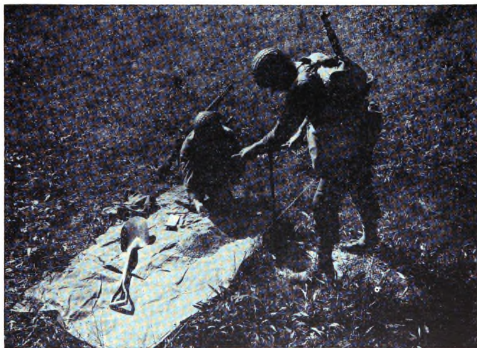
Figure 28. Soil survey. Sinking test hole with auger. Soil is classified, data is recorded on profile sheets (fig. 29), and samples are saved.
